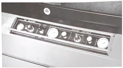
◆An air over oil hydraulic tensioning and tracking system is used to provide rapid belt changes and the ability to alter belt tracking while the belt is running.
