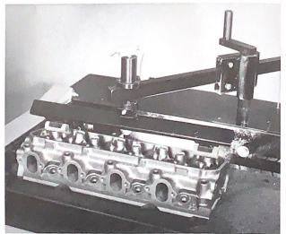
◆The air hold down is standard equipment because down pressure is imperative to obtain maximum abrasive belt life.
