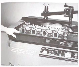
◆ For operator safety there is a fold down fence in front of the work area. For normal operation the fence is in its up position, but it folds down to accommodate work that hangs over the front of the platen.
