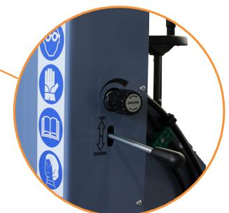
Swivelling cylinder head cradle by handwheel •
