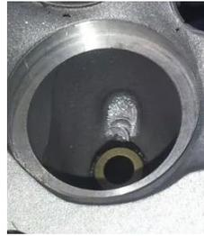
Cam bucket bore machining
