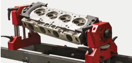
Heads with tilted or canted valve guides can be positioned quickly, even if sides are parallel or not. Set the cylinder head at the desired level and roll it over. Sturdy clamping thanks to two large jaws. Firm locking of the jaw's shafts through two handles for a perfect clamping while machining.
