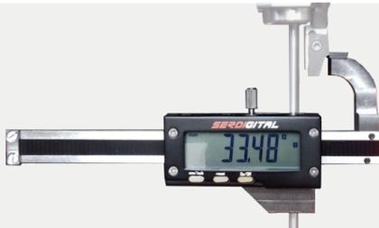
Direct diameter reading digital micrometer. The tool diameter can be easily read and set into the machine control. Values displayed in metric or imperial.
